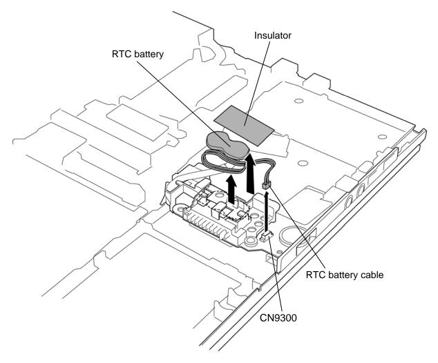
Figure 4-28 Removing the RTC battery
